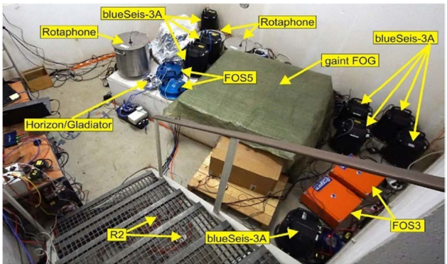
Bild 7 Experiment “Rotation and strain in Seismology: Acomparative Sensor Test“, Geophysical Observatory Fürstenfeldbruck, Germany: rotational sensors mounted in the bunker [6]
