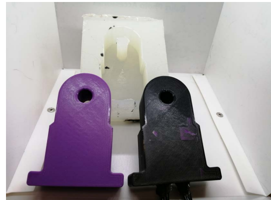
Figure 7 Photo of the 3D printed sensor housing (purple), the silicon based casting mold and the sensor inside the housing.
