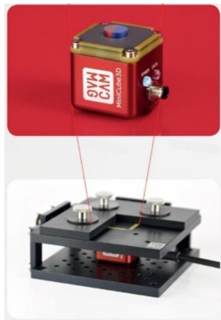
Figure 2 2-pole axially magnetized cylinder magnet measured with MiniCube3D magnetic field camera
