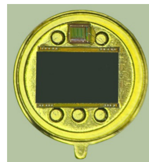
Figure 3: 60 x 40 thermopile array chip mounted onto a TO-5 type header (left), assembled with an IR optics (center) and a thermal image taken with it (right).
