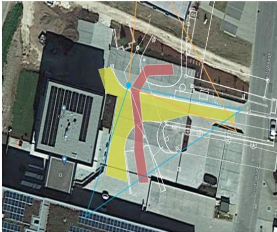
**Fig. 1:** Smart city campus test site plan of ZDE in Westhausen. The red area represents a cycle-foot path and the yellow area represents a street / Underground parking garage entrance. The blue- and orange line triangles indicate the visible areas of the observing cameras. (This figure was created by ZDE and contains material from Google.)
