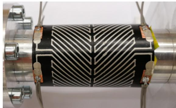
Fig. 9: Fabricated sensor element.
