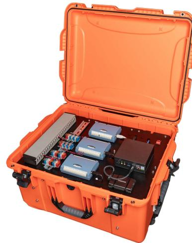
*Figure 3: Hardware setup of a DisDAQ system inside a watertight housing for outdoor usage.*
