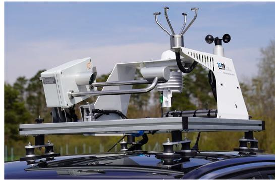
Figure 4: Sensor setup for roof-top installation of the mobile environmental sensor rack (MESR) using a mobile DisDAQ instance.
