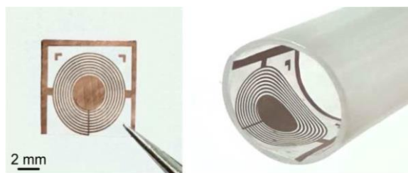
Figure 4: (a) The fabricated results. (b) The pressure sensor attached on curved surfaces.
