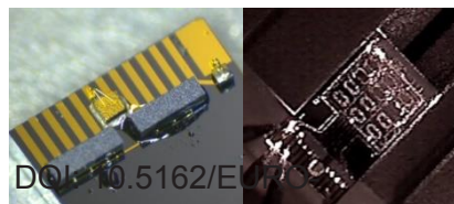
Figure 1. (1) Bialoom PIC on stage – size 25mm x 25mm; (2) PHOTO-SENS PIC with VCSEL, photodiodes and NTC thermistor on chip – PIC size 3mm x 5 mm.
